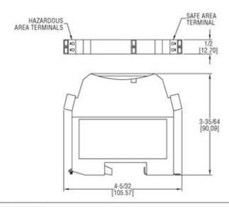
The ENVIROMUX-ISZB Zener Barrier is an intrinsically safe shunt-diode barrier that can be used to communicate with and provide isolations for certain transmitters approved for use in hazardous areas. These barriers limit the amount of energy allowed to pass into the hazardous area, which inhibit ignition in flammable atmospheres.
