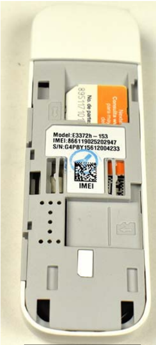
4- Slide SIM card into slot fully. (Card is fully in slot above)
