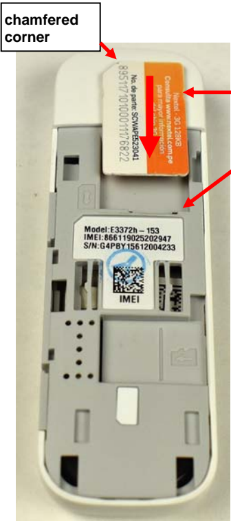
3- Set SIM card on modem above card slot. The chamfered corner is at top left.
