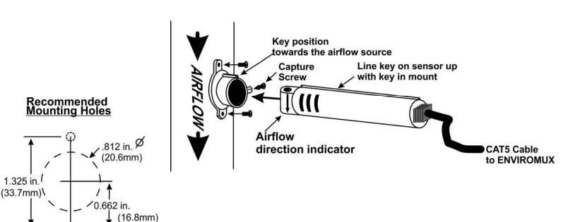
.125 in.Ø (3.18mm) The sensor can be mounted at any depth, but for best performance position the sensor such that the opening in the sensor body is in the center of the airflow chamber. The body of the sensor will allow for centering in a chamber as deep as 11 inches when using the mounting adapter provided.
