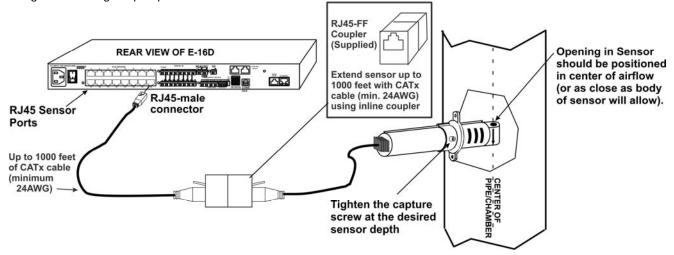
WARNING: To avoid damaging the E-AV-LC-7 Air Velocity Sensor, it should only be operated where it will sense at least some air flow ( $\geq$  8.2 ft/s (2.5 m/s)) daily.
