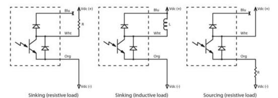
The NPN output is electrically isolated from the DC power inputs and case. The NPN output may be externally connected to the same supply as the DC power inputs or to a different supply.
