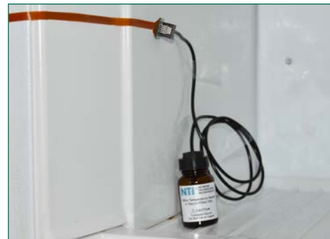
E-FW-1 - Flex Wire is used to connect E-T1WGM-xx to E-1W without interfering with the refrigerator/freezer seals.
